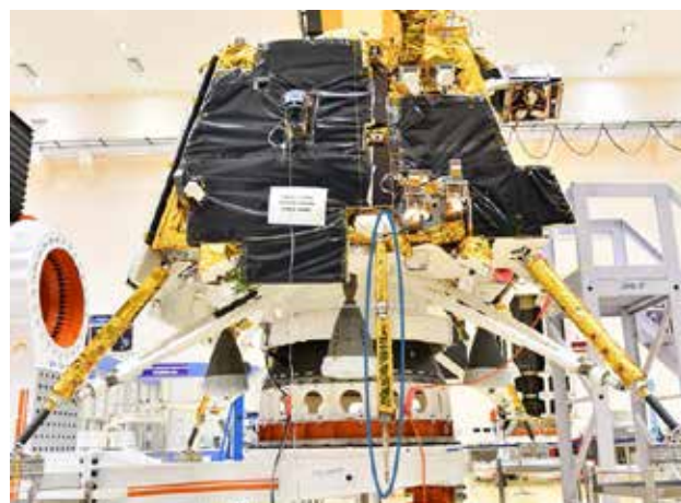
Figure 1: ChaSTE probe deployment and penetration operations as part of the IST
