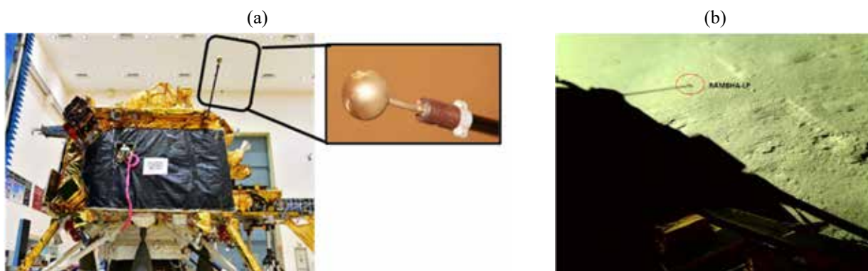
Figure 13: (a) Photograph of RAMBHA-LP system during Spacecraft level Deployment & Functional Test. (b) The photograph the Chandrayaan-3 lander, showing the shadow of the deployed LP.
