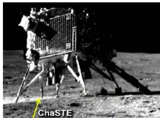
Figure 15: The photo of Chandrayaan-3 lander taken by the rover camera. ChaSTE is seen in the inserted configuration.
