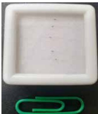
Figure 16: A pack of five thermistor sensors (small dots inside)
