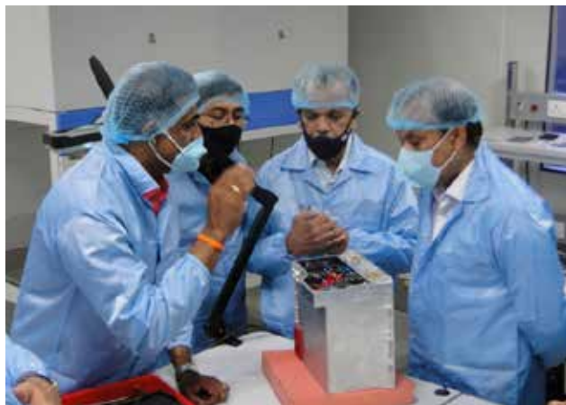
Figure 10: Assembled PAPA payload (FM) in the clean room
