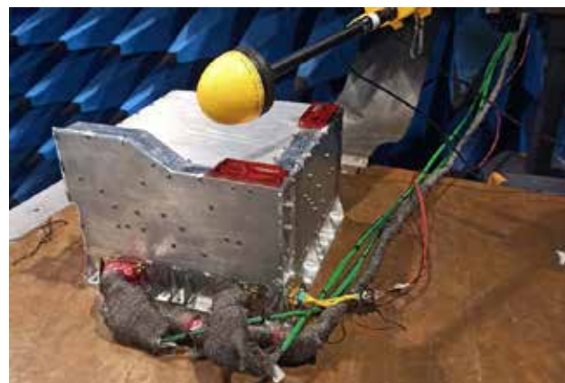
Figure 5: EMI/EMC test setup of the PAPA payload (proto-FM)
